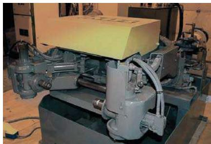
We use only the best quality brass alloy with the high content of copper. The reliable system of gravitational molding of bodies ensures the highest quality of molding, absence of micropores and stress in the metal.
