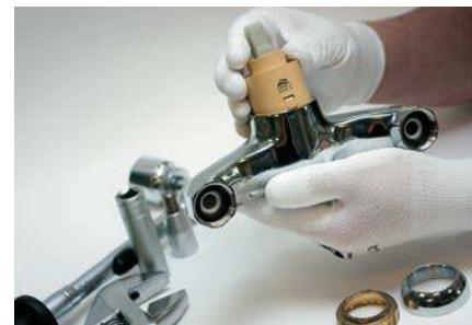
**Assembly.** Some elements (cartridges, valves) require the verified and correct assembly with a certain force of a clip. For a guarantee of firm assembly without damage of the parts, we use dynamometric wrenches. Such attention to the process ensures durability of all components of the faucet.
