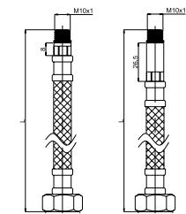
**M10xF1/2" stainless steel wire, EDPM rubber (short nozzle)
