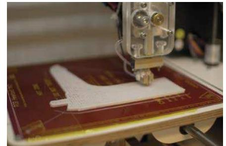
At the following stage the model of the faucet is produced with the help of 3D printer. In this way we can test line of the design and check for design errors.
